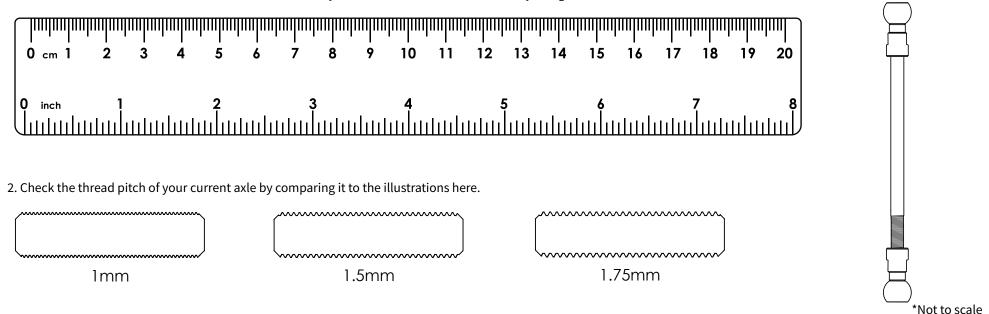
3. Measure the length of your current axle using this illustration. Measure to the end of the threads.
