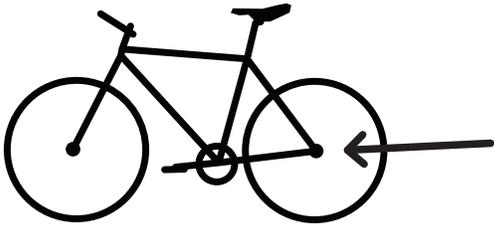
The axle is located here. It goes through the rear wheel of the bicycle.
